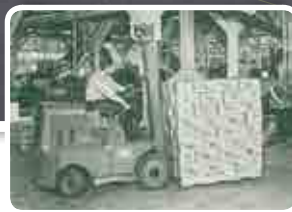
The Carloader is introduced. It is the world's first modern short-coupled, internal combustion forklift truck.
