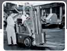
The industry's first nested I-beam upright is produced by CLARK. This upright design dramatically improves upright strength, load stability, and visibility.
